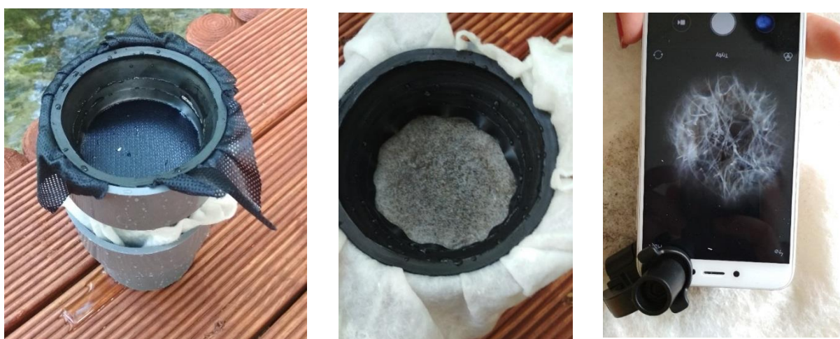
Fig.1. The equipment for microplastics collection and monitoring
